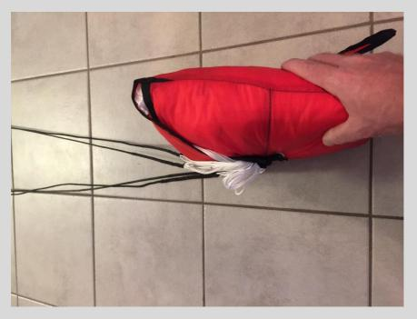
Twist the container 180° counterclockwise (direction of rotation, if you look in direction of the harness) and if the reserve parachute will be installed on the right side of the harness. Otherwise opposite.
