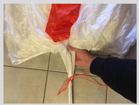
For easy packing, you may install a packing rope to bundle the lines.
