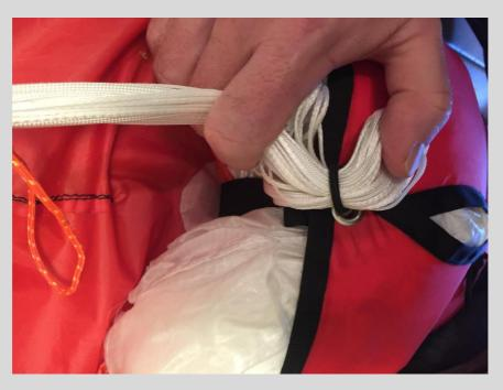
Take the rubber loop and both leaves of the container and close it with the bundle of lines.
