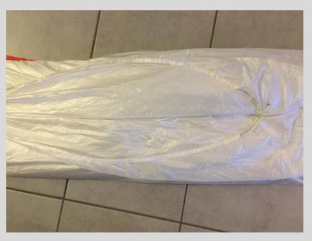
Position the rear tip on the top of the wound-up panels and open the gap. This special and easy packing method guarantees a much faster opening as the standard S-fold.
