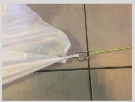
The DIAMONDcross has only one packing loop. This is sufficient for easy packing of the canopy and saves time. The loop is aligned with the tension stripe on which the red front tip is also connected.
