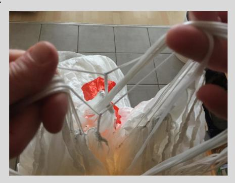
Continue and check that all centerlines are between the two front and two rear fork lines. CAUTION: If the center lines are not between, there is a line over and the canopy is inside out.
