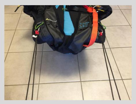
Install only approved connectors with at least 500 kg WLL (Work Limit Load). If you use Dyneema links, install them according to the instructions of the manufacturer.
