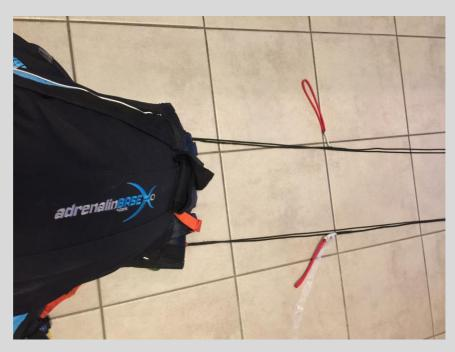
Turn harness in clockwise direction (rotation direction if you look in direction of the canopy). Attach harness, so that it is possible to apply tension during packing
