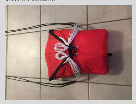
The redundant loops to close the container prevent an inadvertent or too early opening during the extraction of the container from the harness.
