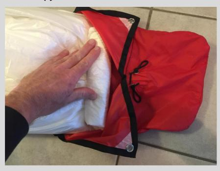
Wind-up approx. 10 - 15 cm of the top of the canopy and put it into the bottom of the inside container.
