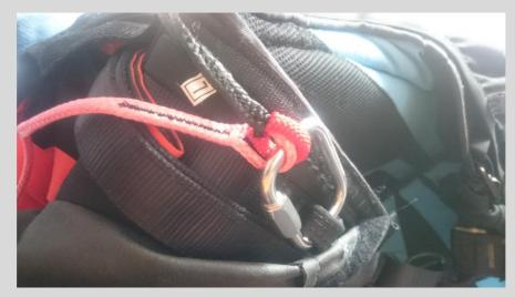
Connect riser and red safety connection with "L" or "Left" to left hand side (flight direction) of the harness. Connect RH riser and red safety connection to right side of reserve parachute attachment point of the harness. **Put both loops on each side into the shackle!**
