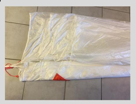
Fold panels two times at approx.1/3 of depth in direction of the center. You may use packing clamps or weights.
