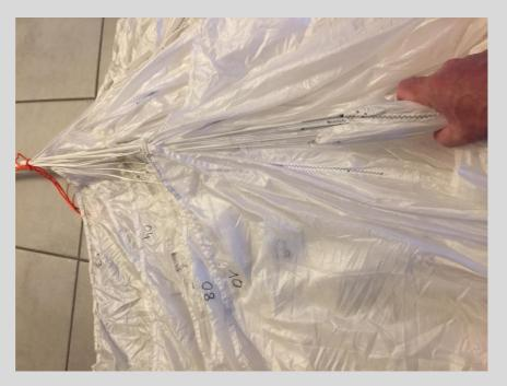
Align the center lines in the middle of the canopy. Pull to tension the center lines and move the material of the canopy in the center up as far as you can reach inside for better folding in the next steps.
