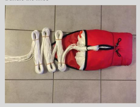
Position the lines according the picture and bundle the lines with three loops on each side of the bundle.
